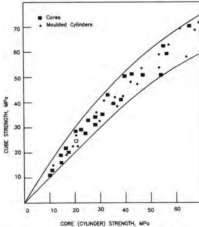
Fig. 3.3.1. Cube/Core (Cylinder) Strength Relationship<sup>3</sup>
