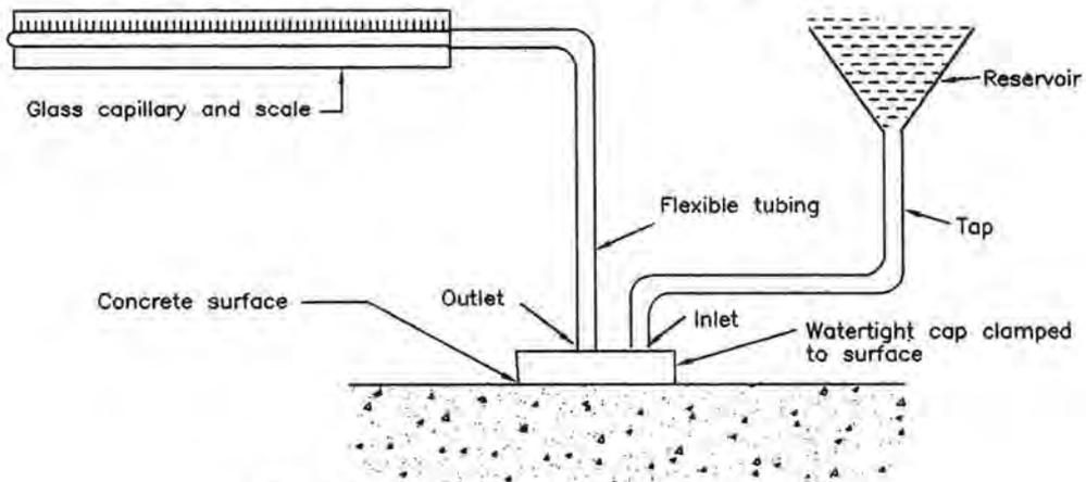
Fig. 3.11.1. Initial Surface Absorption Test<sup>11</sup>
