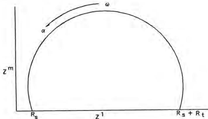
Fig. 3.34.2. Nyquist Plot for Steel in Concrete
