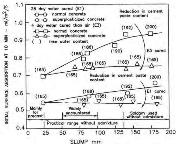
Fig. 3.11.7. Effects of Concrete Slump on its Initial Surface Absorption<sup>80</sup>
