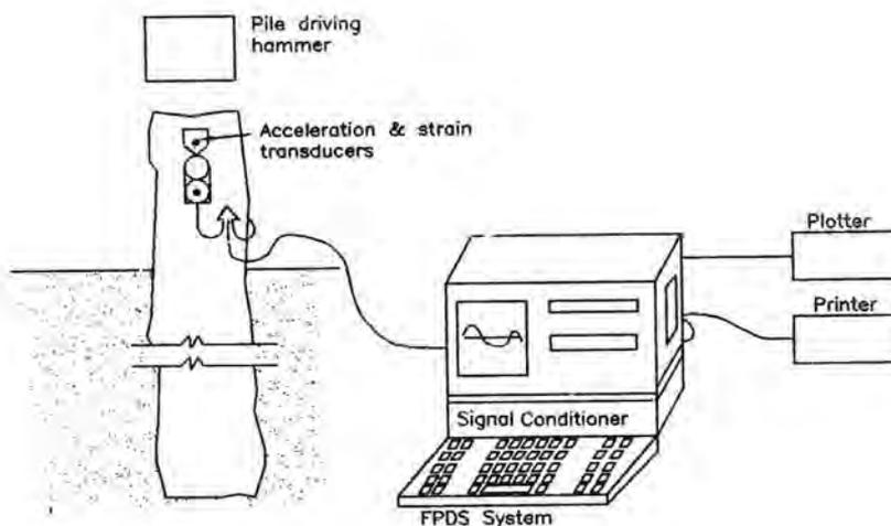
Fig. 3.39.4. System Concept for PDA/DLT<sup>157</sup>
