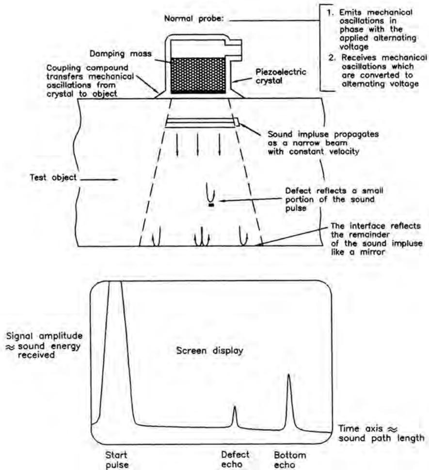
Fig. 3.10.1. Principle of Ultrasonic Examination<sup>87</sup>
