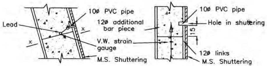
SECTION SHOWING FIXING OF EMBEDDED TYPE V.W. GAUGES
