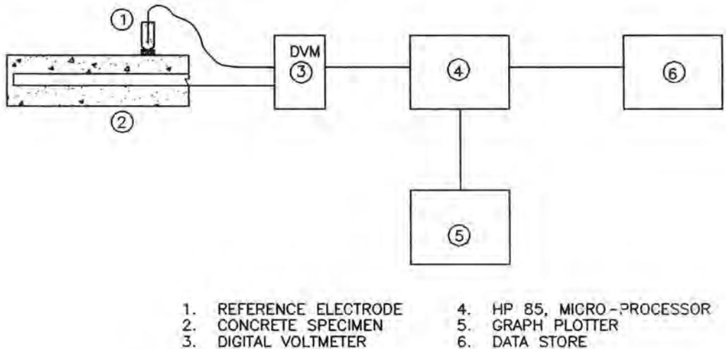
**Fig. 3.35.1. Block Diagram of Noise Measuring Instrumentation**
