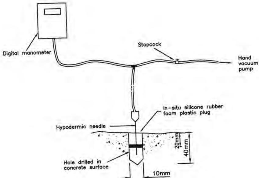
Fig. 3.12.1. Modified Figg's Air Permeability Test<sup>11</sup>
