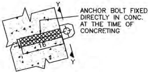
SECTION SHOWING FIXING OF S.S. ANCHORS FOR V.W. STRAIN GAUGES
