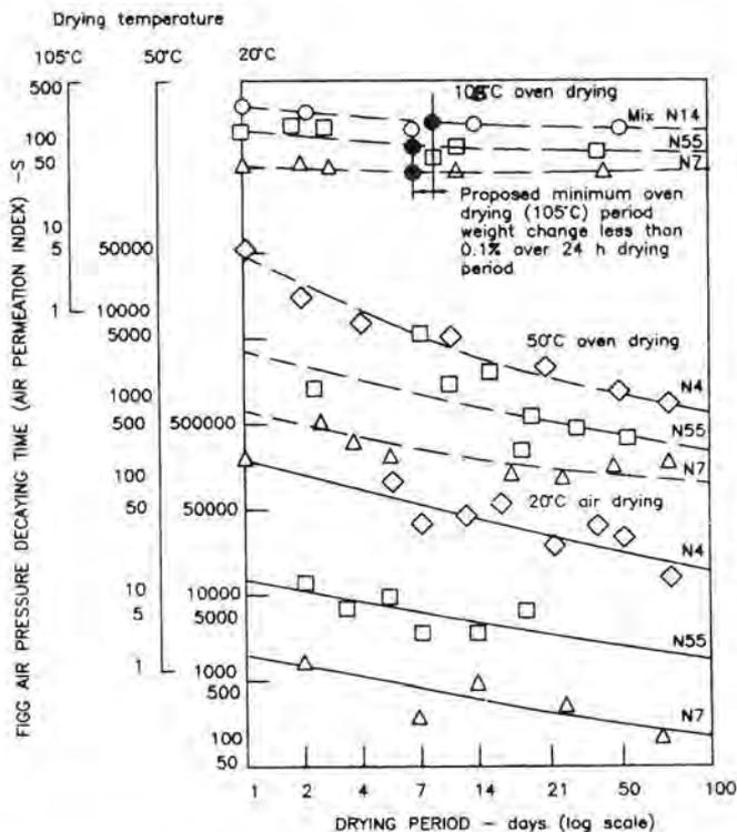
Fig. 3.12.2. Relationship between Air Permeation Index and Duration of Drying<sup>80</sup>
