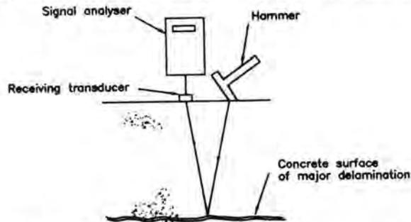
Fig. 3.10.2. Instrumented Delamination Device<sup>11</sup>
