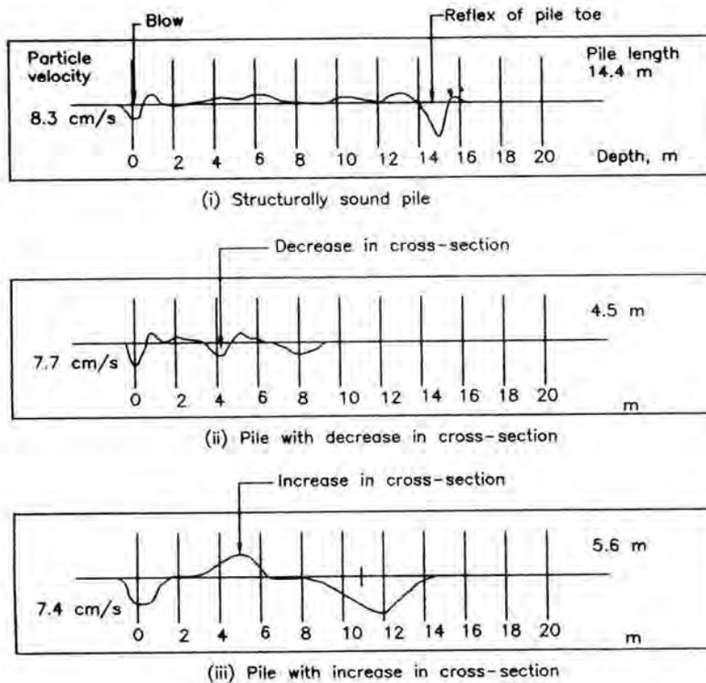
Fig. 3.39.3. Typical Integrity Test Results<sup>155</sup>
