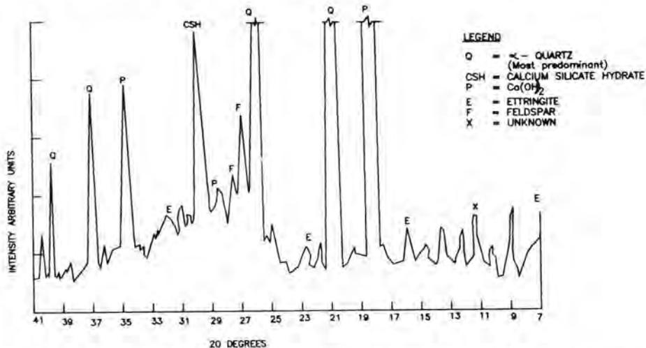
Fig. 3.17.1. X-ray Diffraction Pattern of an Old Hardened Concrete Sample
