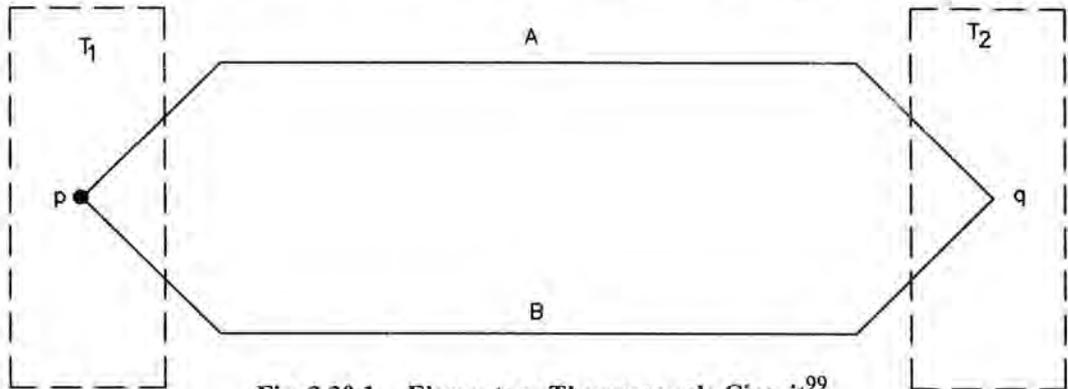
Fig. 3.30.1. Elementary Thermocouple Circuit<sup>99</sup>
