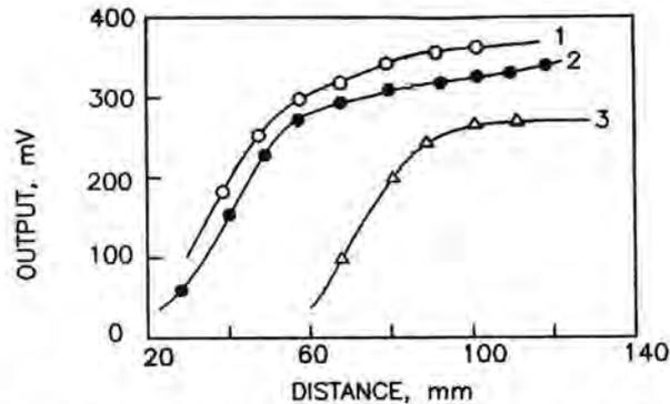
Fig. 3.22.1. Relation between Cover Thickness (distance in mm) with Output Voltage (mv)<sup>5</sup>
