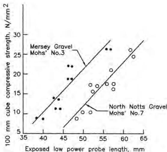
Fig. 3.2.2. Typical Low Power Calibration<sup>1</sup>
