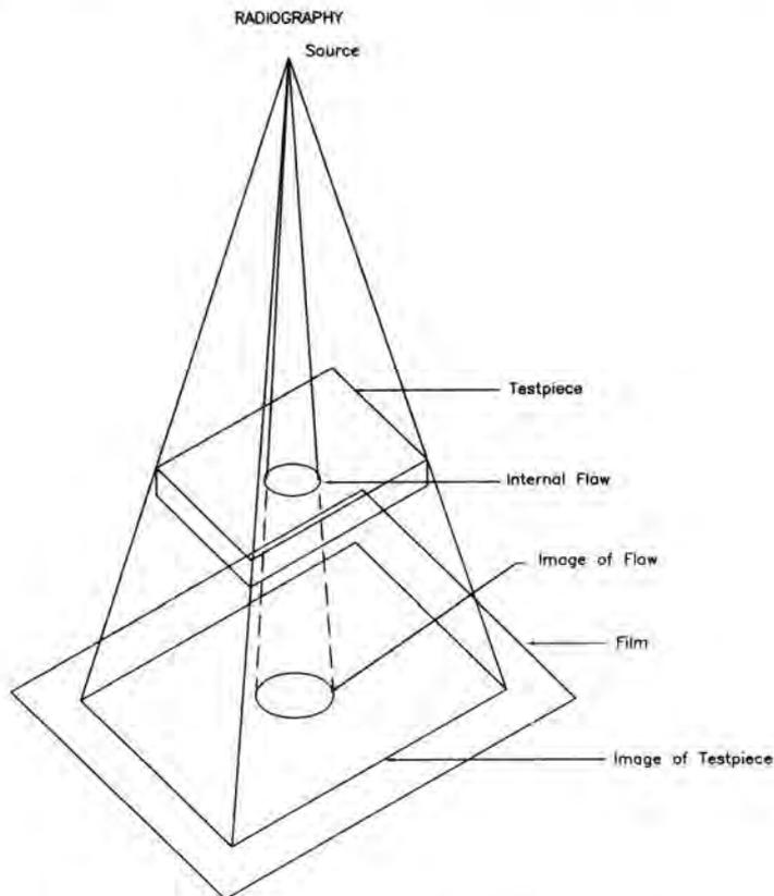
Fig. 3.19.1. Schematic Diagram showing Radiographic System<sup>90</sup>
