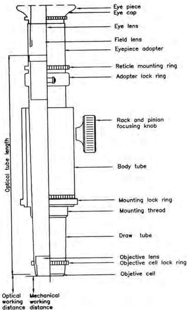
**Fig. 3.20.1.** Section through a Simple Low-Power Microscope<sup>99</sup>
