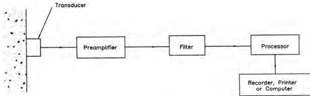
Fig. 3.9.1. Acoustic Emission Equipment<sup>11</sup>
