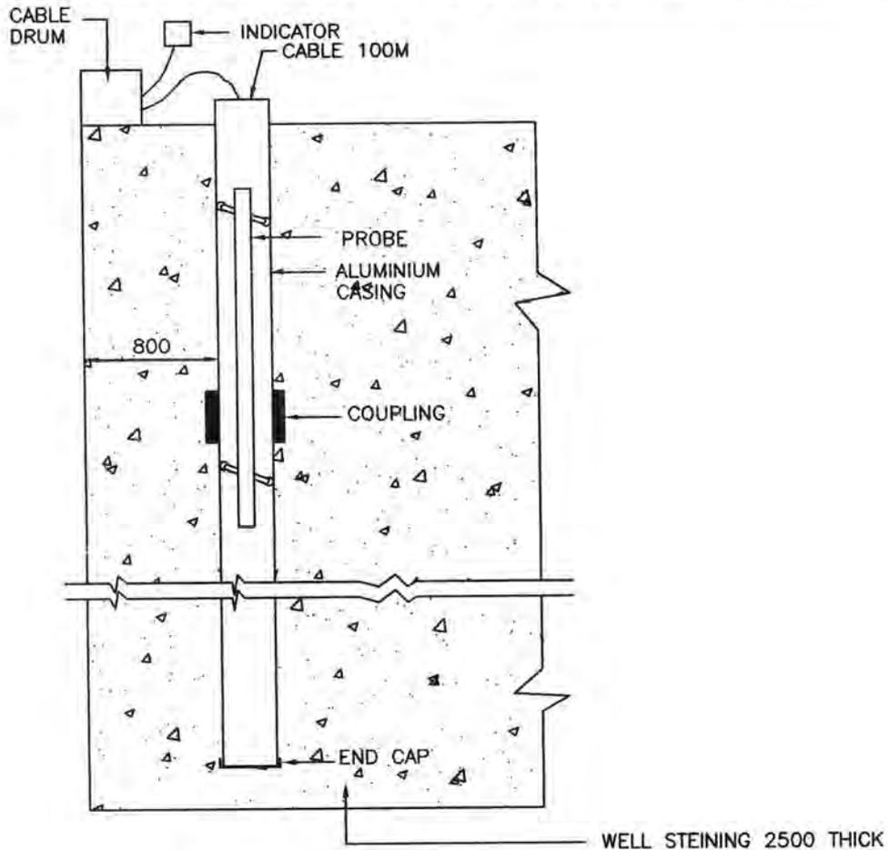
**Fig. 3.28.1. Inclinometer System (Schematic)<sup>169</sup>**
