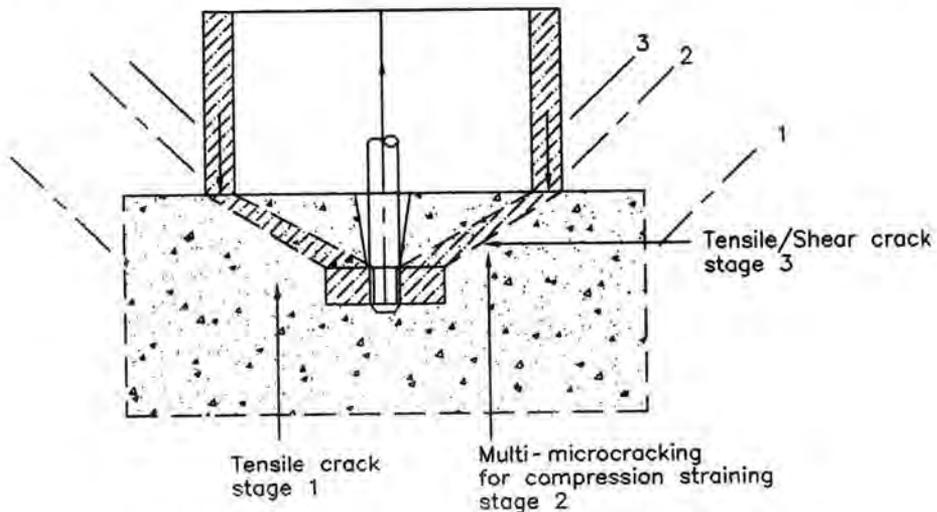
**Fig. 3.4.3. Internal Cracking Stages during a Pull-out<sup>153</sup>**
