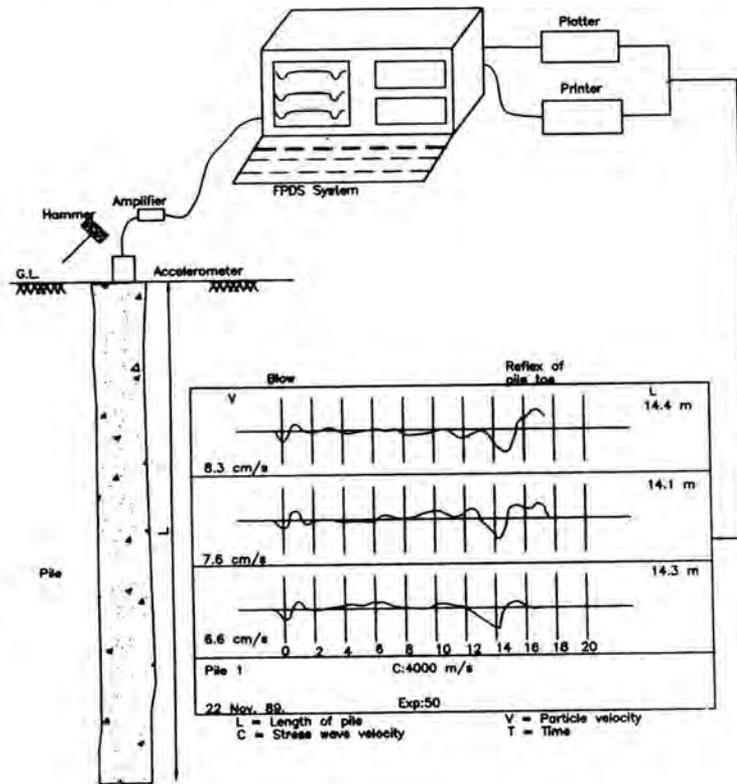
Fig. 3.39.1. System Concept of Integrity Test<sup>158</sup>
