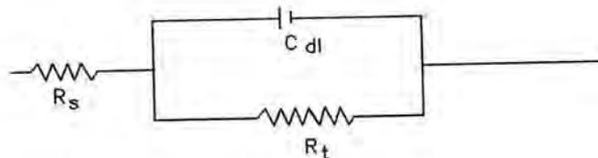
**Fig. 3.34.1. Equivalent Circuit of a Corroding Rebar Embedded in Concrete**
