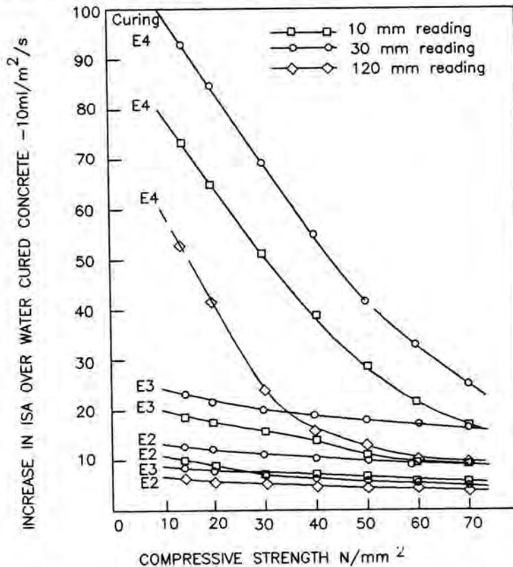
Fig 3.11.6. Influence of Concrete Grade on the Increase in ISA under various Curing Conditions with respect to Water Cured Concrete<sup>80</sup>
