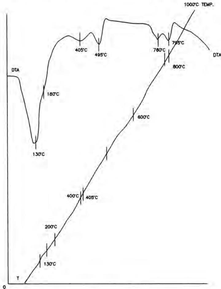
Fig. 3.17.2. DTA Graph of an Old Hardened Concrete Sample
