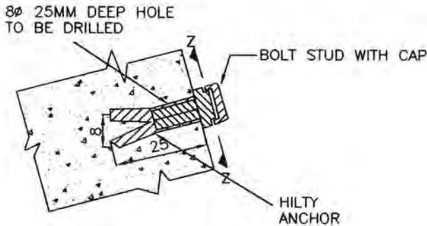
SECTION SHOWING FIXING OF BOLT STUDS FOR MECHANICAL GAUGE
