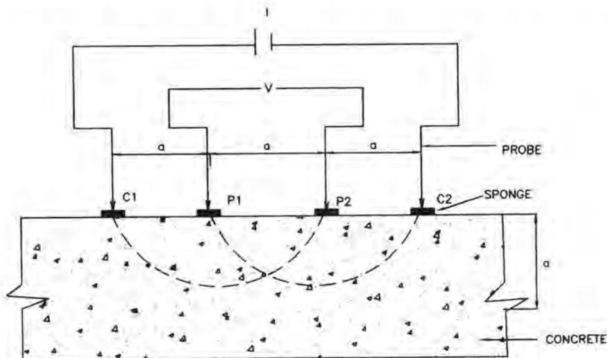
Fig. 3.36.1. Circuit of FPR Meter
