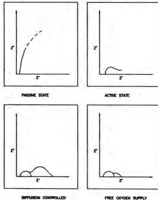
Fig. 3.34.3. Typical Impedance Plots
