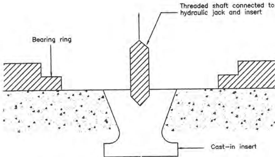
Fig. 3.5.1. North American Pull-out Method Assembly<sup>1</sup>
