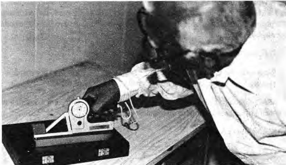
Fig. 3.26.L. Pfender Gauge held on Standard Bar
