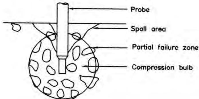
Fig. 3.2.1. Compression Bulb Produced by Penetration Probe<sup>1</sup>
