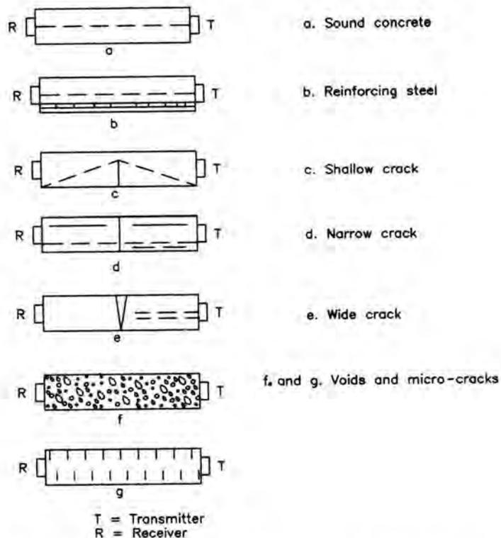
**Fig. 3.8.2. Factors Affecting the Transmission of Sound Wave through Concrete<sup>8</sup>**
