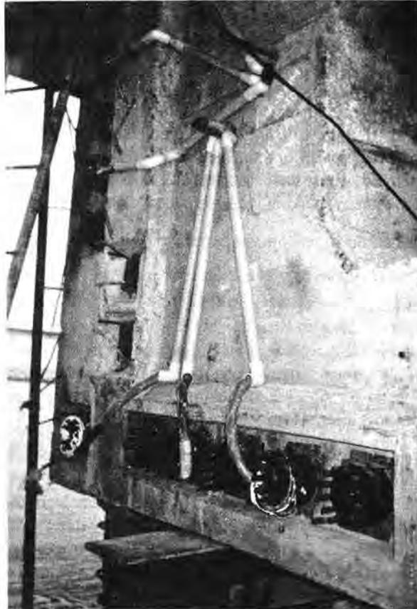
**Fig. 3.38.1. Various Arrangements for Cable Resistance Measurements**
