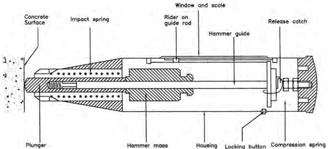
Fig. 3.1.1. Typical Rebound Hammer<sup>11</sup>
